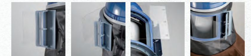
The lens for KD-509 is easily replaceable by the unique lens replacement mechanism using the levers attached to the goggle part.
